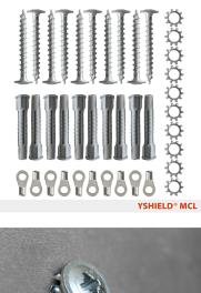
**Grounding set for the use with our magnetic shielding film MCL61.** The MCL61 surface is electrically insulated. Whilst screwing down the cable lug, the chopper disks will perforate the polyester film and arrange electrical contact thereby.
